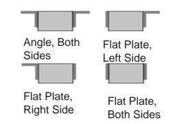
Bumpers may be ordered with angles or flat plates at each end. Use a flat plate for mounting bumper next to a dock leveler, or where the space is to tight to allow the use of angles. Note: When using the flat plate, it is welded to the dock.
